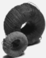
The world's first ferrite core
