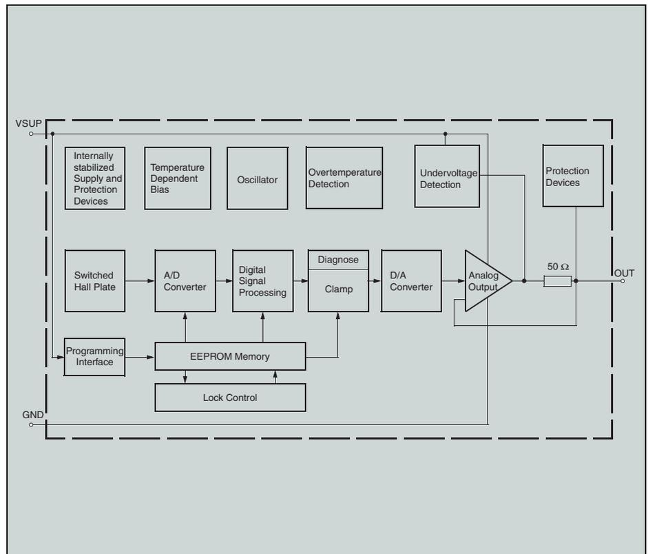
Fig. 2: Block diagram of the HAL 1880
