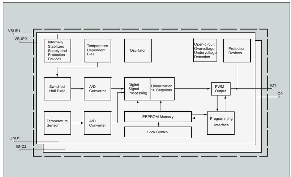
Fig. 2: Block diagram of the HAR 2455 with PWM output
