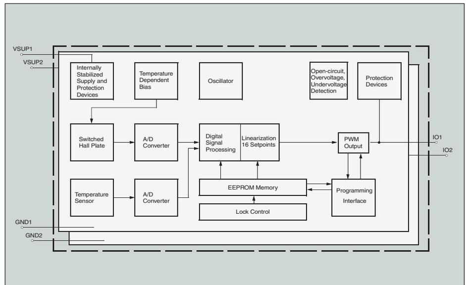
Fig. 1: Block diagram of the HAR 2425 with ratiometric analog output
