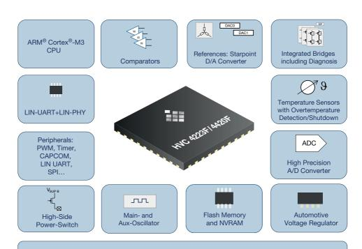
Functional Safety Support, ISO-Pulses, AEC-Q100, LIN 2.x conform, EMC conformity according to worldwide OEM Specifications, ESD (8 kV @ LIN Port), −40 °C ≤ T<sub>.I</sub> ≤ +150 °C
