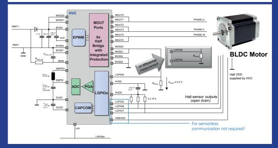
Stepper Motor Current Control. Motor currents driven by internal MOSFET bridge. For continuous motor currents up to 500 mA.
