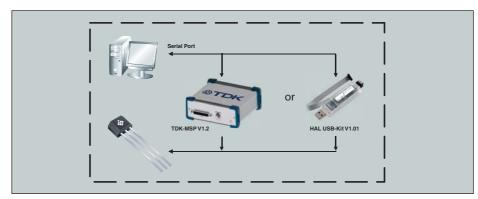
Fig. 1: Development tool setup for HAL 18xy
