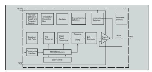
Fig. 2: Block diagram of HAL 1880
